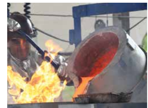
Molten brass pours into the Marine Aviation Memorial Tower's bell cast
